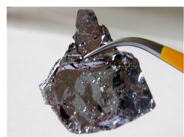
Figure 1: A hexagonal piece of MoS2 with a lateral size of 15- x 20mm
